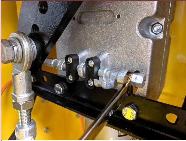
Disengage the gearbox with a 10mm spanner to allow free movement of the spring arm.
