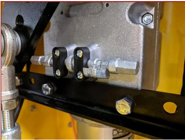
This image shows the gearbox disengaged
